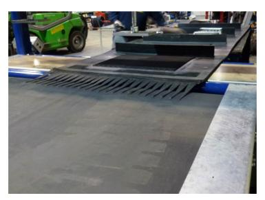
The Belt Feeder-Work-Bench has a conveyor belt incorporated for the transport of the ready bonded profiles on the belt.
