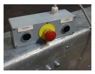
Operation is easy with the handheld, with the buttons 'Hold-to Run' and an emergency button.
