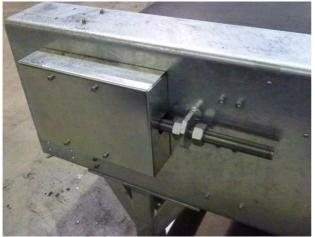
The tension system for the conveyor belt.
