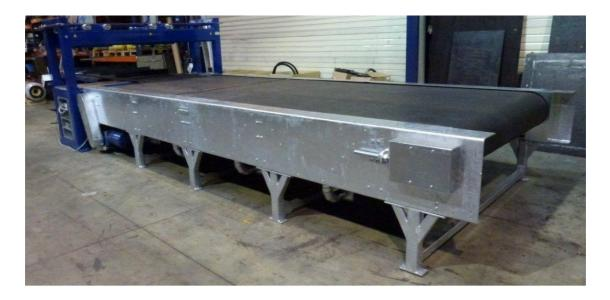
The ICE-Trade Belt Feeder-Work-Bench is conceived for two reasons; one is that the gases during the cold bonding process are sucked away by the special developed suction system and second to 'feed' the <a href="ICE-Trade Profile Press">ICE-Trade Profile Press</a> in case conveyor belts are made with cleats and or sidewalls.
