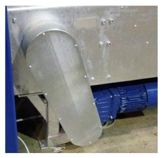
As a conveyor installation the Belt Feeder-Work-Bench has an engine / gearbox. The secondary drive is a duplex chain.
