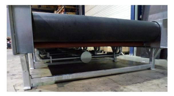
The ICE-Trade Belt Feeder-Work-Bench features a gas suction system, for the gases from the bonding cement. Per section the suction system can be opened or closed, which is depending the length of the belt to be made and the length Work-Bench.
