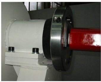
Winders fitted with **Safety Chucks**.
