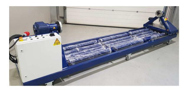
The ICE-Trade Belt Winders are produced according the specs of the customer: the width, diameter, weight of the belts and the needed power. Our standard winders feature a variable winding speed till 10 m/min.
