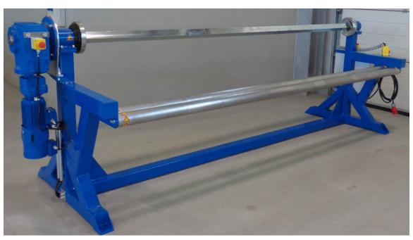
For steering the belt ICE-Trade developed a simple and efficient system, so that the conveyor belt can be reeled neat. The ICE-Trade Steering System is offered as an option.
