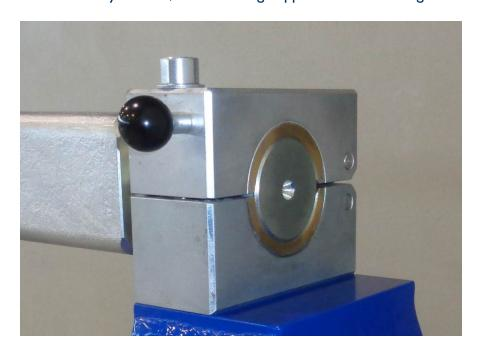
In case the Brass Bearing Support is installed the ICE-Trade Coupling connects the winding axle with the gearbox.
