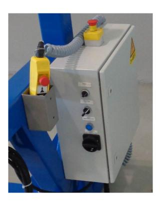
Operation of the belt winder is with a handheld or foot pedal which is 'hold-to-run'.
