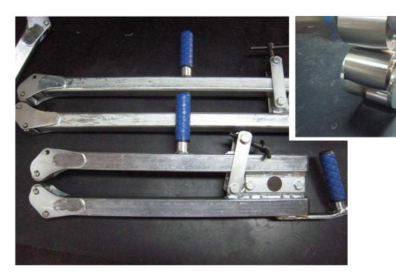
The ICE-Trade Double Pressure Rollers for rolling the cold bonded splice of the conveyor belt. The ITDPRs are electro galvanized and features stainless steel rollers, with bronze bearings.
