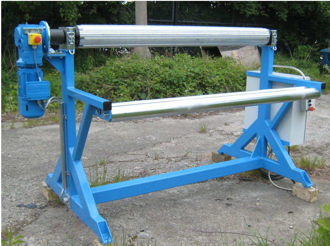
ICE-Trade multiple Strip / Sheet Winder with ICE-Trade Coupling and Brass Bearing Support
