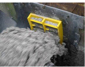
Depending the contact surface of the material hitting the chute 1, 2 or more Protectors are installed in the chute.
