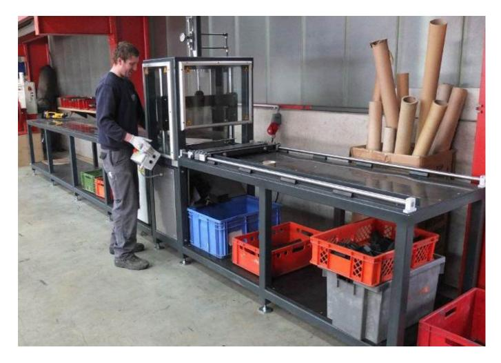
The ICE-Trade Guillotine for Cleats is developed to cut cleats, quick, safe and rational. The ITGC features an input table and output table, made to size according the request of the customer, a stopper to cut all the cleats on the same pre-set length, a removable cover next to the knife to have the smaller size cleats slide in a box under the table and is covered at the top with "security" glass.
