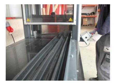
Smaller cleats can be cut multiple, as the knife has a length of 500 mm. The knife is made from high quality HSS.
