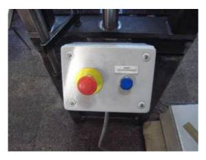
Furthermore the control box features the emergency stop and reset button for the emergency circuit.
