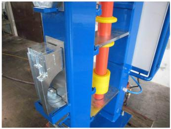
Storage of the roller base, support & press plates is at the side of the frame.
