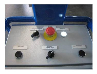
The control box features on/off switch, emergency stop system, switch for the positioning, switch up/down, and the two hand operating buttons which have to be pushed synchronic.
