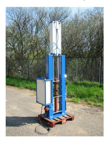
The ICE-Trade® Rubber Ring Press presses the buffer and support rings on the roller. The first ITRRP is launched in April 2011.
