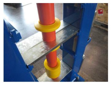
The roller base, press and roller support plates are galvanized.
