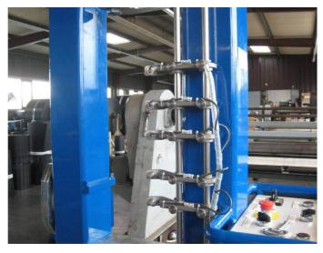
Sensors ensure the right positioning of the rings on the idler.
