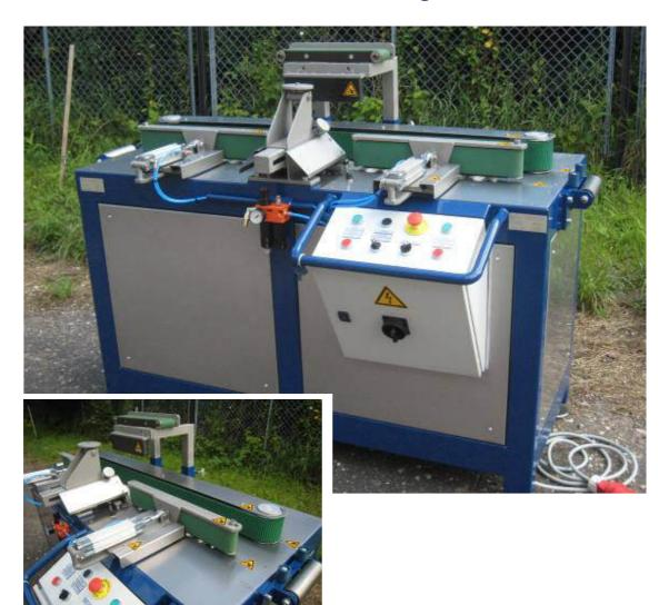
The ICE-Trade Sidewall Buffing Machine, ITSwBM, is developed to grind the bases of the sidewalls. The ITSwBM can buff sidewalls from S 40 till S 400.
