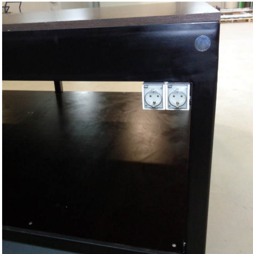
Work Bench detail with 22 mm thick work blade (multiplex plywood) and plugs for the power tools
